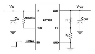
The output voltage is calculated by:
