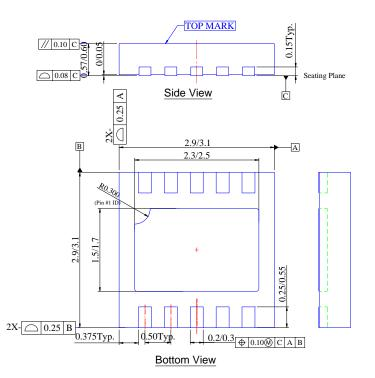
Note: 6. ALL DIMENSIONS ARE IN MILLIMETERS. ANGLES ARE IN DEGREES. 7. COPLANARITY APPLIES TO THE EXPOSED HEAT SINK SLUG AS WELL AS THE TERMINALS.
