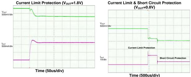
Short Circuit Protection (Vout=1.8V) Short Circuit Recovery (Vout=1.8V) V<sub>OUT</sub> 500mV/div V<sub>OUT</sub> 500mV/div **Current Limit Protection** I<sub>OUT</sub> 500mA/div Short Circuit Protection I<sub>OUT</sub> 500mA/div Time (50us/div) Time (2ms/div)
